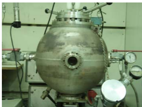
Fig. 3 The 20 L spherical explosion vessel (20-L-Apparatus) for this study
